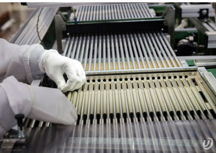
Pellet loading into fuel rods
